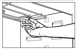
■ Unscrew the nut and lower the Browning / Broiling element.
