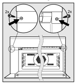
■ Open the door and use the screws supplied to secure the oven to the side walls of the cabinetry through the holes in the oven trim.
